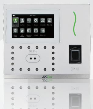
**G3** Pro is powered by latest Computer Vision Technology for proactive facial recognition, which means the terminal can perform bio-authentication with a user's facial attributes as soon as the sensor detects a face.
